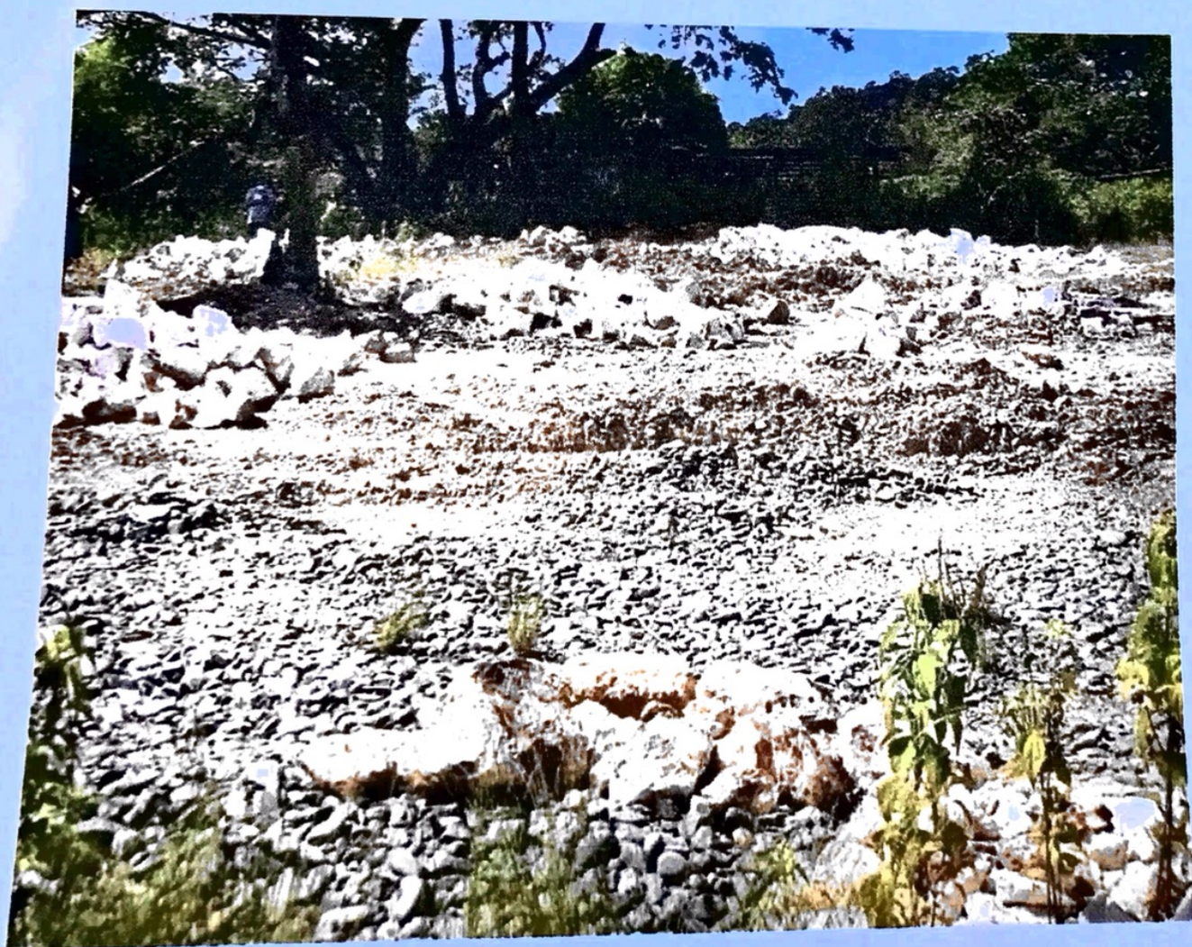
This photo shows the pervasive exposure of a portion of the surveyed quarry area for siliceous rock materials. The rock sizes range from cobble to boulders. Vegetation is composed of tropical grasses and several stunted trees.
